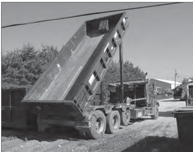
Roll-offs (also commonly but erroneously called dumpsters) are rectangular boxes with wheels that allow the containers to be easily pulled off or on to tracks for hauling away waste. Image courtesy of the author.
