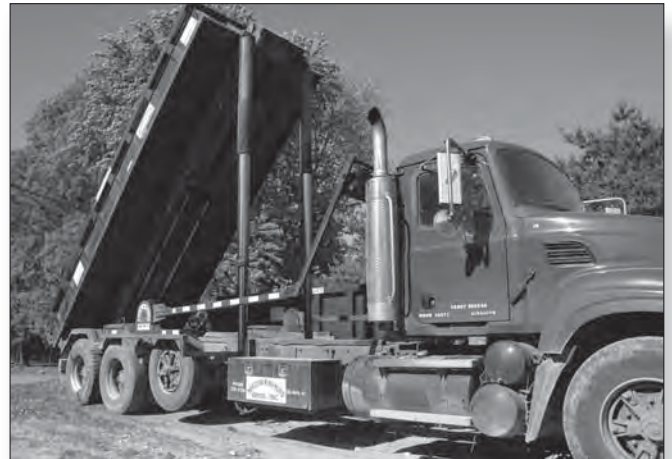
The hydraulic cylinders on a truck used to raise one end of a roll-off for emptying. Image courtesy of the author.
