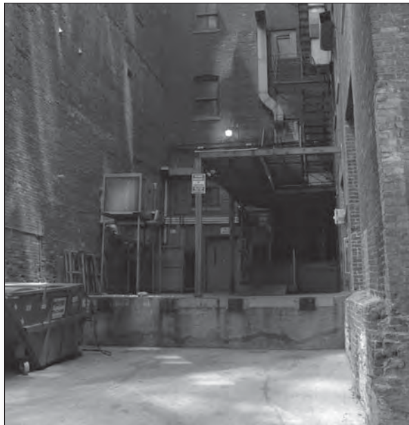
A typical loading dock where new material is delivered and from which waste is hauled away. In front of the dock to the far left is an enclosed waste container that can be loaded onto a truck. Image courtesy of the author.
